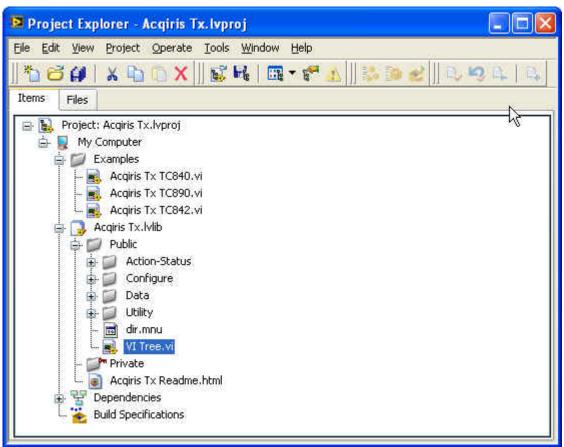
The Example folder contains ready to use potential starting points for your own programs. Individual library functions can be found at the Public level or in one of the 4 categories shown. Query functions are in the Utility folder. The block diagram of the VI Tree.vi can be used to access individual functions. It allows quick and easy access to all needed vi's.
