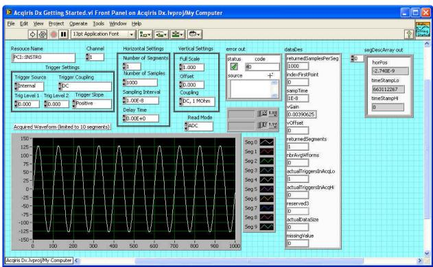
This VI demonstrates how to use some of the basic components of the AqDx Acqiris Digitizer Driver. It finds and initializes a digitizer, sets the basic parameters according to the controls on the front panel, and then acquires one waveform. Note that the front panel controls should be set to their desired values before the VI is run.
