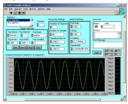
This VI presents a basic, interactive virtual oscilloscope using the AqDx Digitizer Driver. Not all the functionality of the Acqiris digitizers is supported in this program, but most of the most-commonly-used functions are demonstrated in it.
