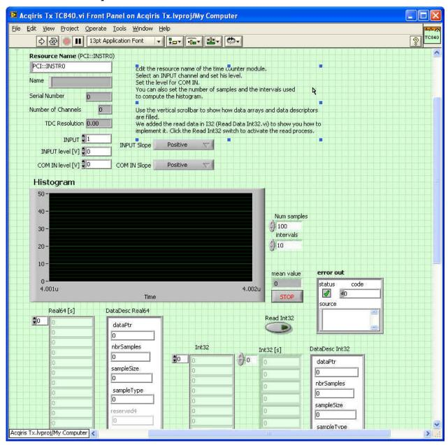
This VI demonstrates how to use a TC840 Time-to-Digital Converter. It finds and initializes an instrument, sets the basic parameters according to the controls on the front panel, and then acquires and accumulates data as the user requests. Note that the front panel controls should be set to their desired values before the VI is run.
