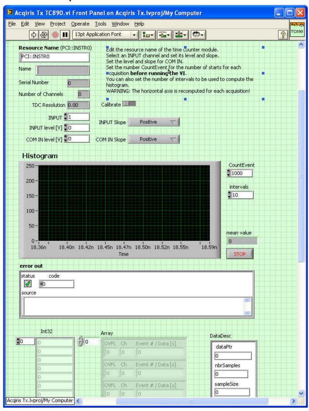
This VI demonstrates how to use a TC890 Time-to-Digital Converter. It finds and initializes an instrument, sets the basic parameters according to the controls on the front panel, and then acquires and accumulates data on the common and the chosen channel as the user requests. Note that the front panel controls should be set to their desired values before the VI is run.
