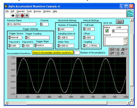
This VI demonstrates how to use the Accumulate Waveform function of the Acqiris Digitizer Driver. It finds and initializes a digitizer, sets the basic parameters according to the controls on the front panel, and then acquires and accumulates waveforms as the user requests. Note that the front panel controls should be set to their desired values before the VI is run.
