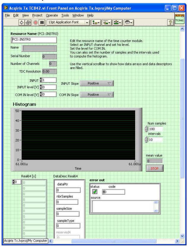
This VI demonstrates how to use a TC842 Time-to-Digital Converter. It finds and initializes an instrument, sets the basic parameters according to the controls on the front panel, and then acquires and accumulates data as the user requests. Note that the front panel controls should be set to their desired values before the VI is run.
